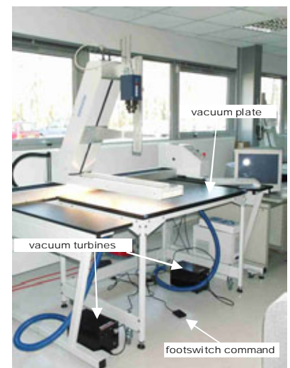
Tests on a vacuum table in the DigiBook production room
